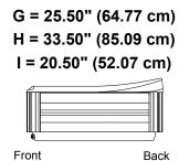
Listed dimensions represent distance from top of acrylic to lowest point in seat. **Tolerance ± 0.5"** (1.27 cm).
