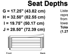
Listed dimensions represent distance from top of acrylic to lowest point in seat. **Tolerance ± 0.5"** (1.27 cm).
